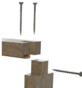
Mortice & Tenon Joint
