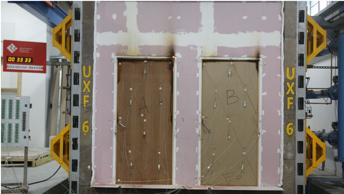
Figure 19 - The unexposed surface of the test construction after a test duration of 33 minutes
