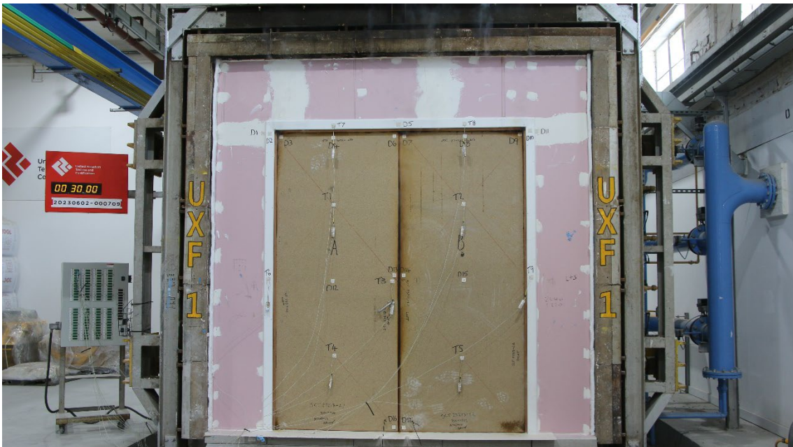
Figure 17 - The unexposed surface of the test construction after a test duration of 30 minutes
