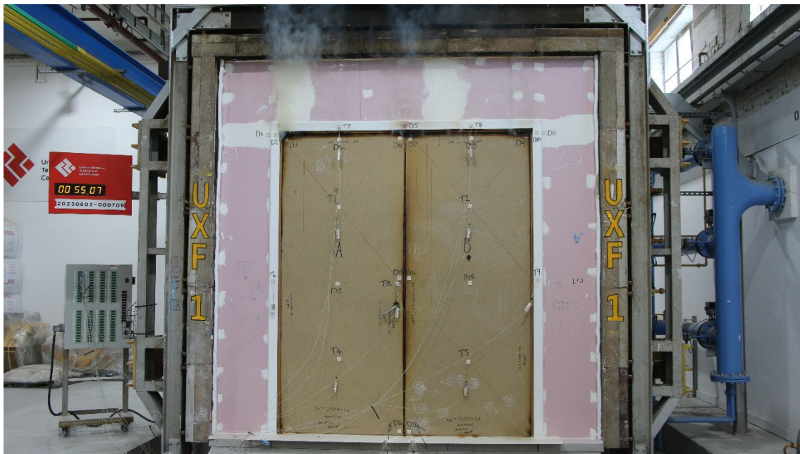
Figure 20 - The unexposed surface of the test construction after a test duration of 55 minutes
