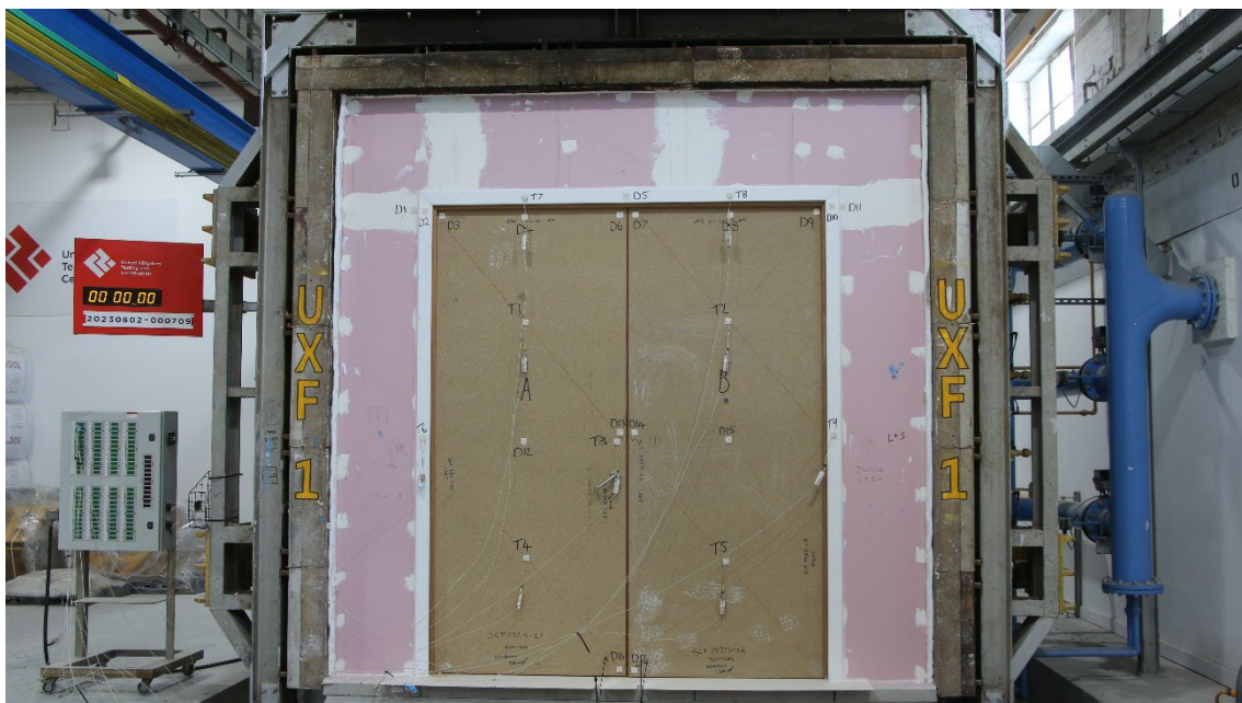
Figure 15 - The unexposed surface of the test construction prior to the commencement of the test
