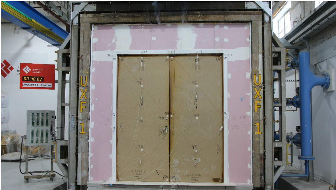
Figure 18 - The unexposed surface of the test construction after a test duration of 40 minutes
