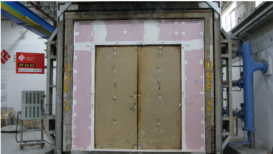
Figure 19 - The unexposed surface of the test construction after a test duration of 50 minutes
