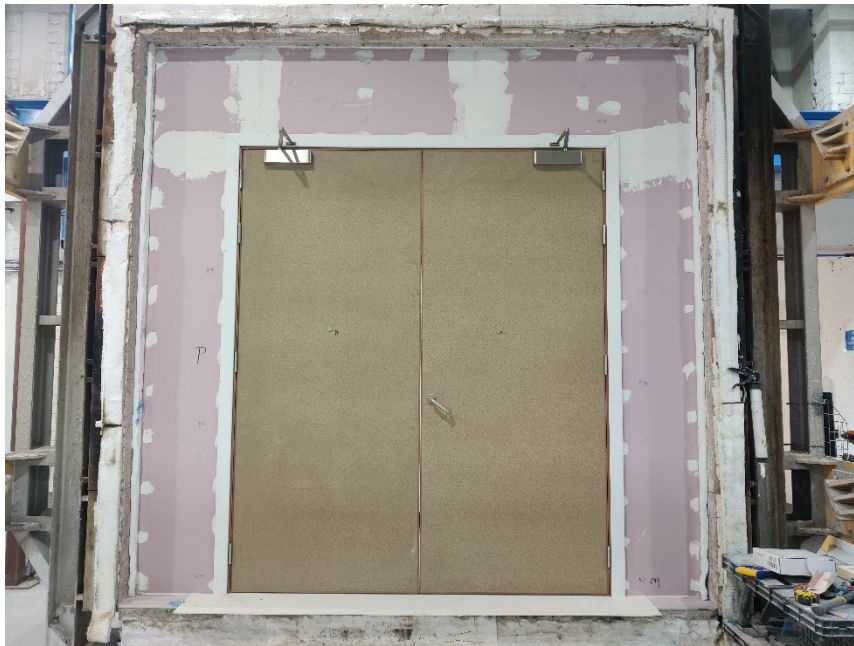
Figure 14 – The exposed surface of the test construction prior to commencement of the test
