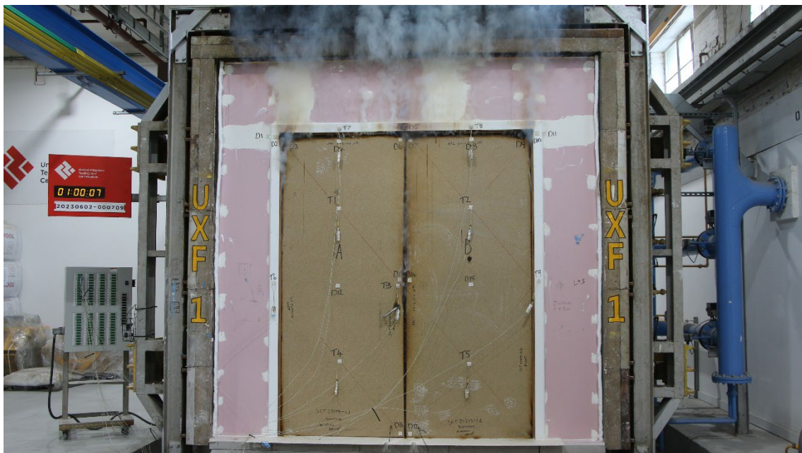
Figure 21 - The unexposed surface of the test construction after a test duration of 60 minutes
