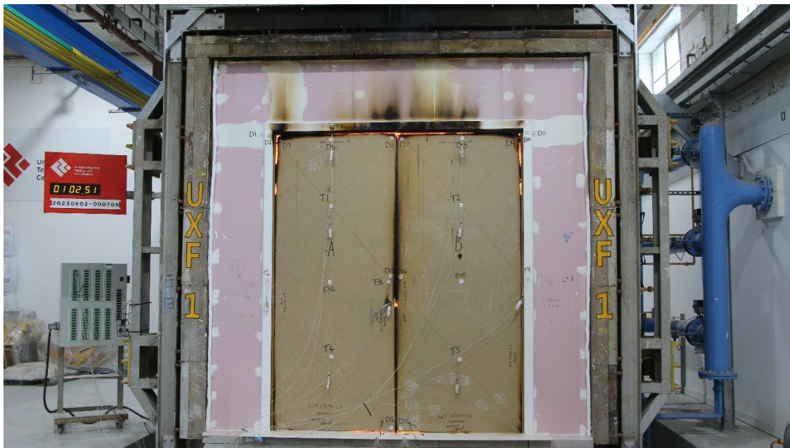
Figure 22 - The unexposed surface of the test construction after a test duration of 62 minutes
