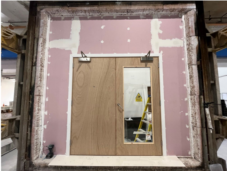
Figure 15 – The exposed surface of the test construction prior to commencement of the test
