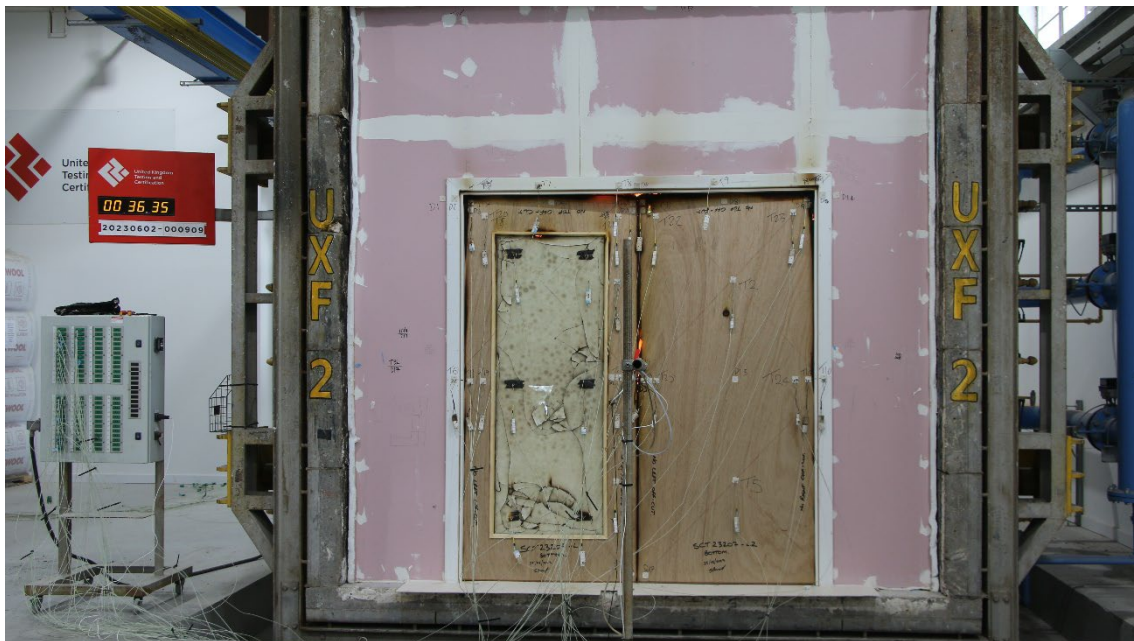
Figure 23 - The unexposed surface of the test construction after a test duration of 36 minutes
