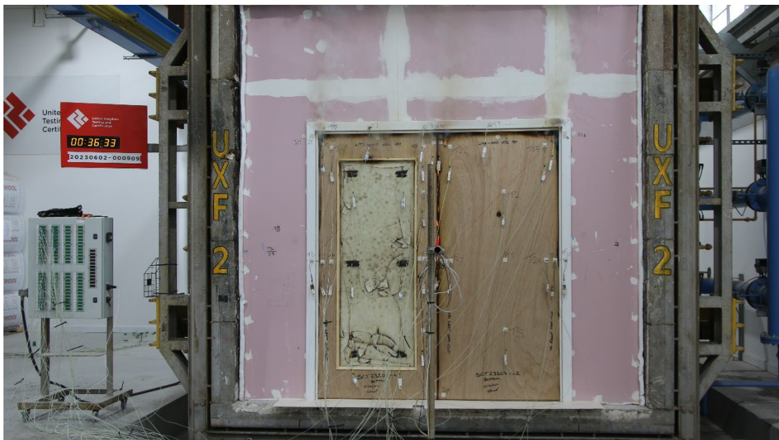
Figure 22 - The unexposed surface of the test construction after a test duration of 36 minutes
