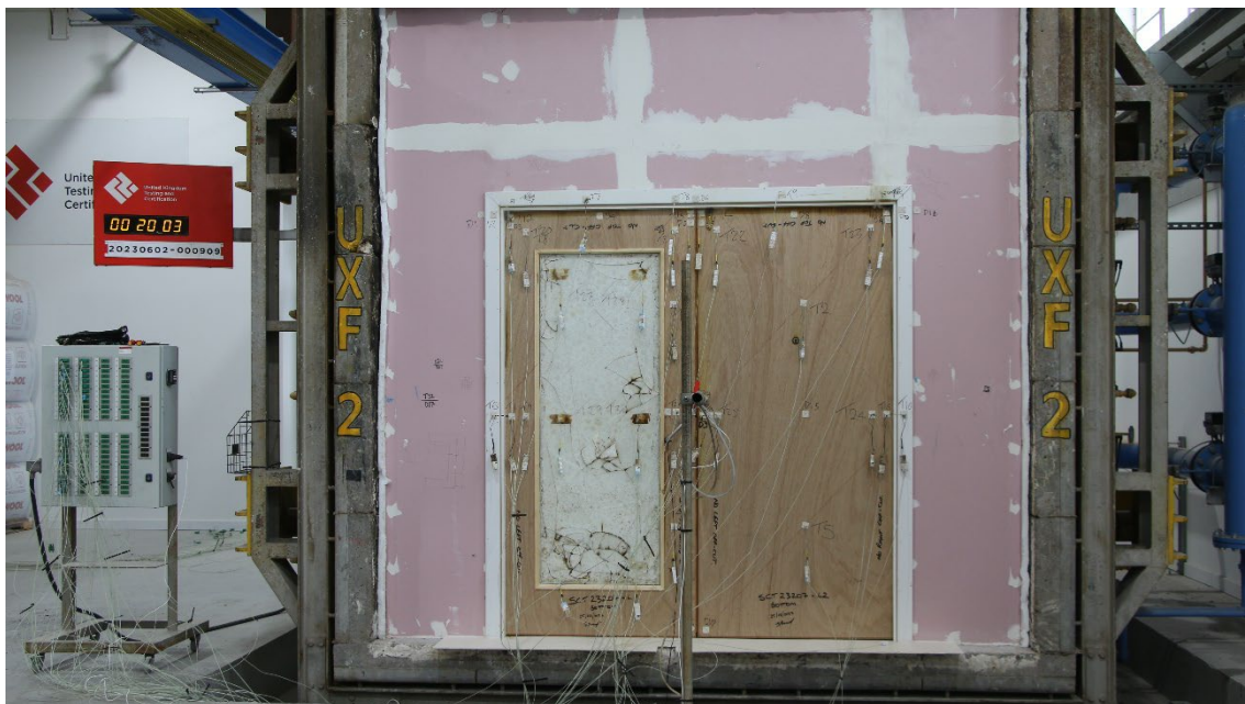
Figure 18 - The unexposed surface of the test construction after a test duration of 20 minutes
