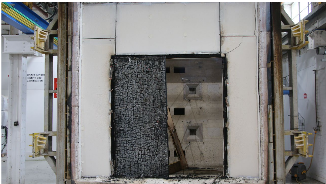
Figure 24 - The exposed surface of the test construction after the test was discontinued
