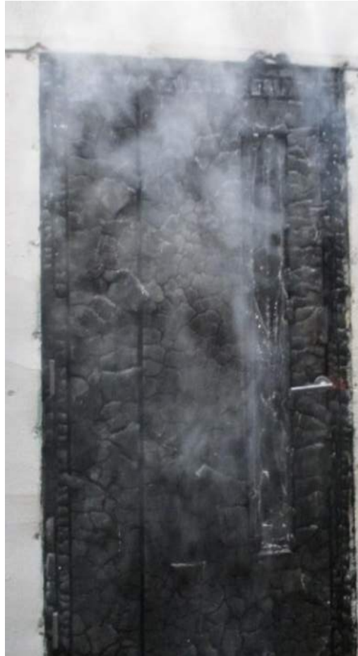
Figure 26 Exposed face of Doorset B at the end of the test
