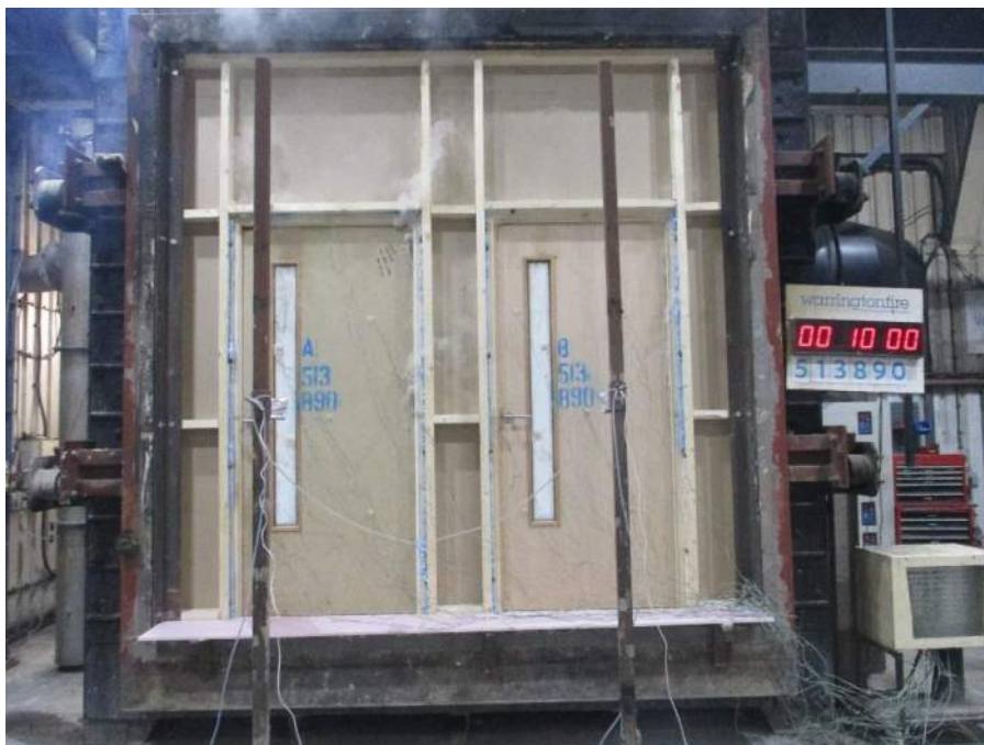
Figure 21 Unexposed face of the specimen after a test duration of 10 minutes
