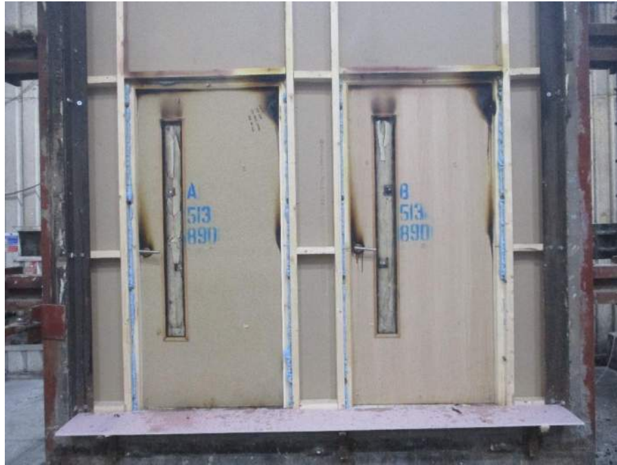
Figure 24 Unexposed face of the specimen at the end of the test
