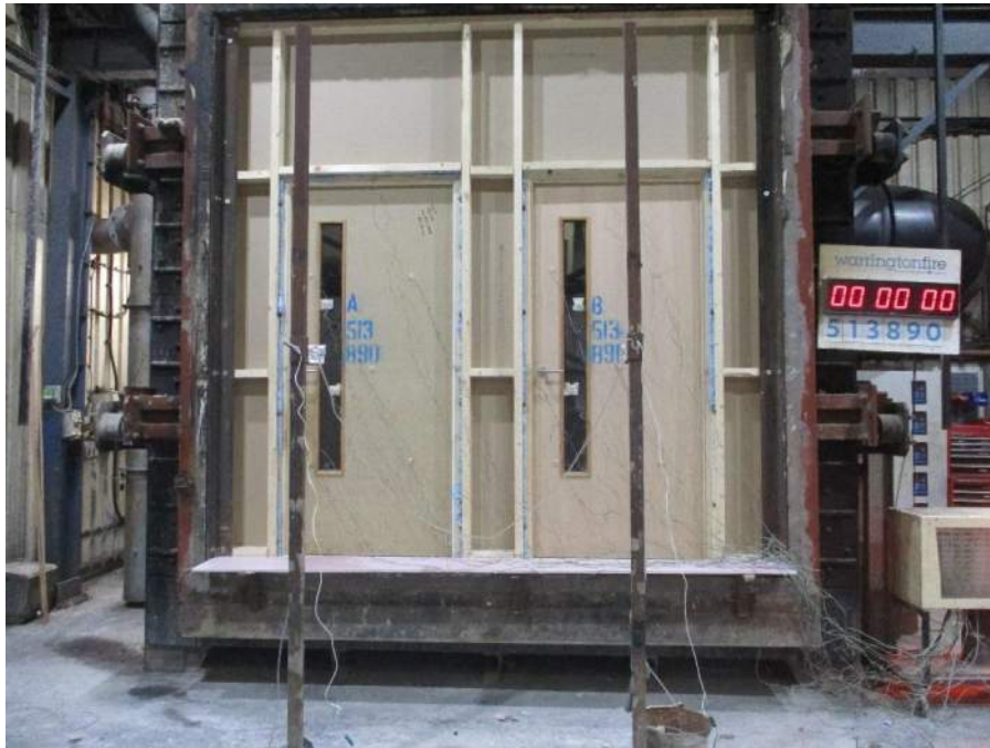
Figure 20 Unexposed face of the specimen before the start of the test
