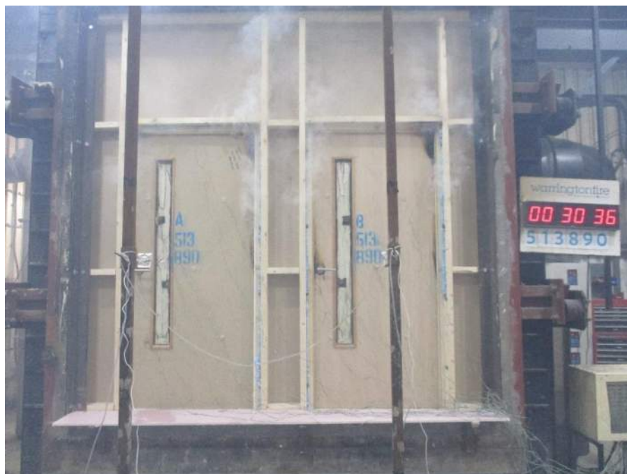
Figure 23 Unexposed face of the specimen after a test duration of 30 minutes 36 seconds
