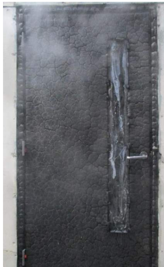
Figure 25 Exposed face of doorset A at the end of the test
