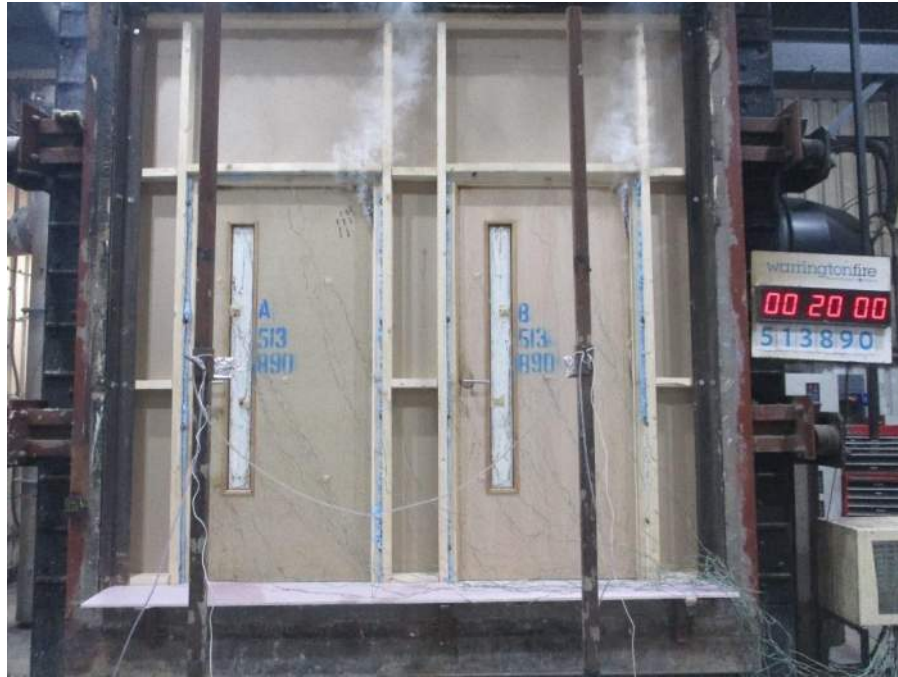
Figure 22 Unexposed face of the specimen after a test duration of 20 minutes
