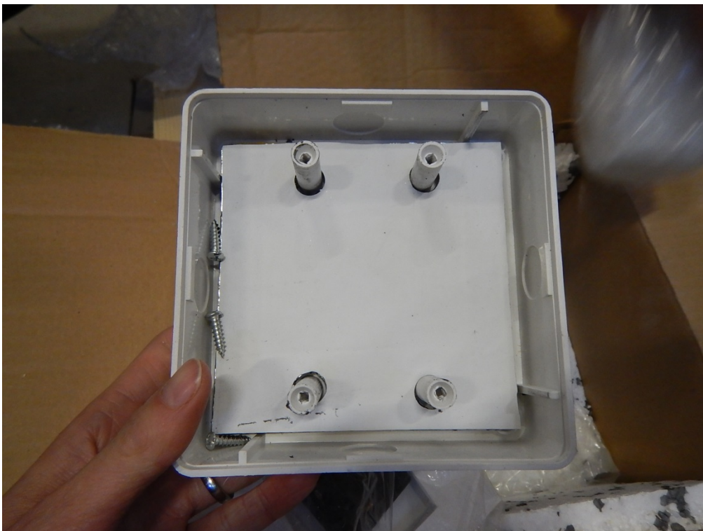
Foto C.6 Detail of the intumescent gasket inside electrical back box
