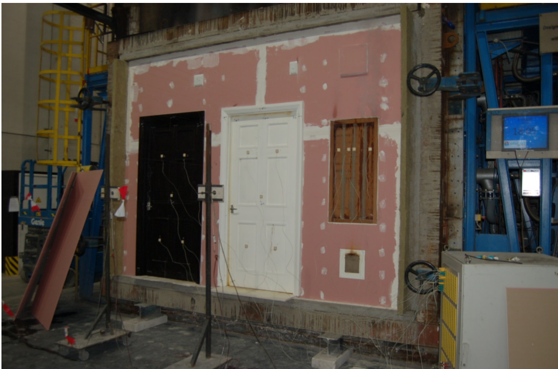
Foto C.10 Specimens after 18 minutes of heating
