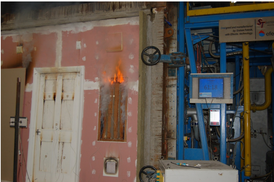
Foto C.14 Specimens after 61 minutes of heating
