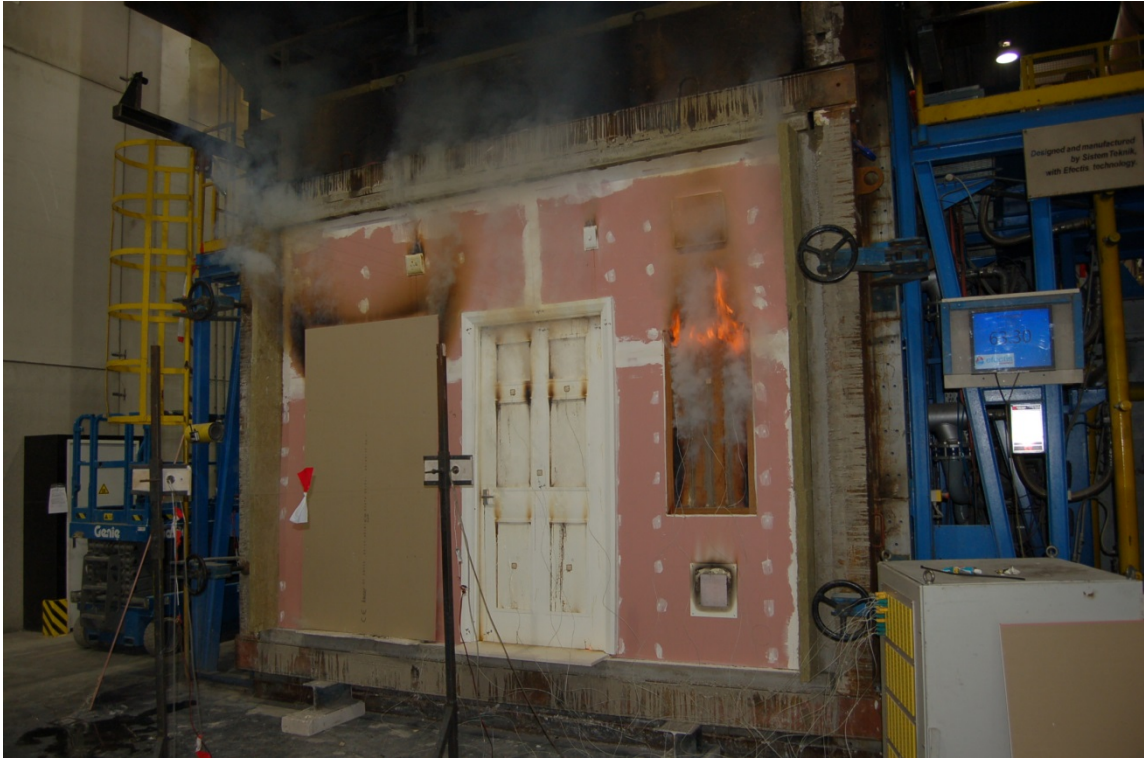
Foto C.15 Specimens after 63 minutes of heating, end of heating after consulting the client
