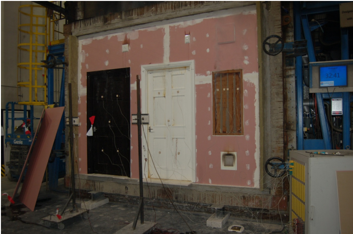
Foto C.11 Specimens after 32 minutes of heating
