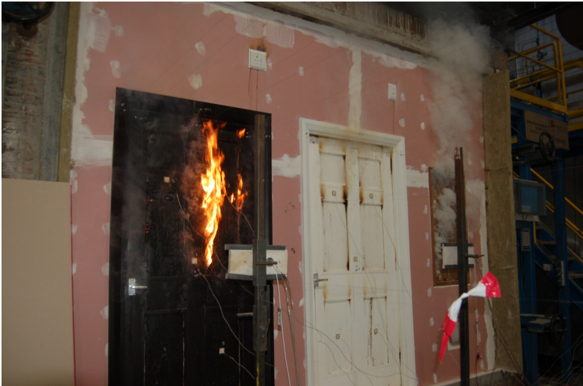
Foto C.13 Specimens after 56 minutes of heating
