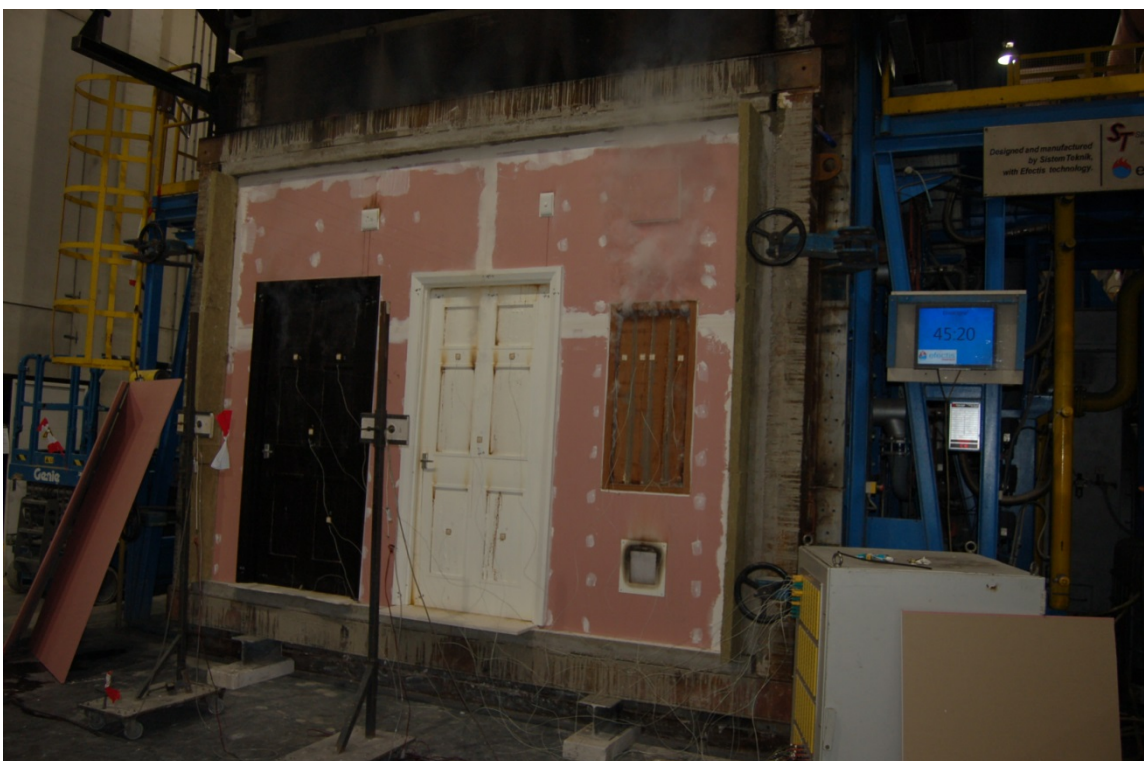
Foto C.12 Specimens after 45 minutes of heating
